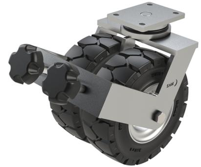
**POA** Fabricated zinc plated twin wheel swivel braked castor with plate fixing fitted with 2x black elastic rubber tyred on a steel disc centred wheel with ball bearings. Wheel diameter 406mm, tread width 2 x 104mm, overall height 484mm, plate size 175mm x 140mm, hole centre's 140mm x 105mm. Load capacity 1900kg at 4kph, 1040kg at 10kph and 860kg at 16kph
