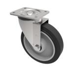
Pressed steel swivel castor with a top plate fixing fitted with a black 65 shore A elastic rubber tyred on cast iron centre with ball bearings. Wheel diameter 200mm, tread width 50mm, overall height 238mm, top plate 135mm x 110mm, hole centres 105mm x 80/75mm and a Load capacity of 500kg at 4 kph 200kg at 10kph, 185kg at 16kph and 175kg at 20kph. REACH compliant also PAH-Free rubber to confirm to EU-directive 2005/69/EC \*\*FOR INTERNAL TOWING ONLY\*\*
