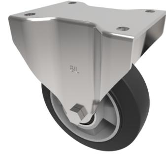
Pressed steel fixed bracket with a top plate fixing fitted with a black high elastic natural 65 shore A rubber tyre wheel aluminium centre with ball bearings. Wheel diameter 150mm, tread width 50mm, overall height 190mm, top plate 135mm x 114mm, hole centres 105mm x 80/75mm. Load capacity 350kg at 4kph and 140kg at 10kph. REACH compliant also PAH-Free rubber to confirm to EU-directive 2005/69/EC \*\* FOR INTERNAL TOWING USE ONLY\*\*
