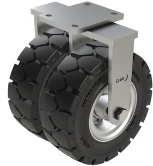
**POA** Fabricated zinc plated twin wheel swivel castor with fixed plate fixing fitted with 2x black elastic rubber tyred on a steel disc centred wheel with ball bearings. Wheel diameter 406mm, tread width 2 x 104mm, overall height 484mm, plate size 175mm x 140mm, hole centre's 140mm x 105mm. Load capacity 1900kg at 4kph, 1040kg at 10kph and 860kg at 16kph
