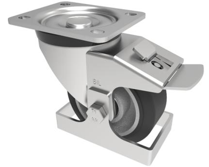
Pressed steel swivel castor with a top plate fixing fitted with a black high elastic natural 65 shore A rubber tyred aluminium centred wheel with ball bearings, total lock brake and footguard. Wheel diameter 100mm, tread width 38mm, overall height 128mm, top plate 105mm x 86mm, hole centres 80mm x 60mm. Load capacity 200kg.REACH compliant also PAH-Free rubber to confirm to EU-directive 2005/69/EC
