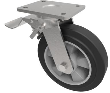
Fabricated white zinc ROHS plated swivel castor with a top plate fixing fitted with a black high elastic natural 65 shore A rubber tyred aluminium centred wheel with ball bearings and total lock brake. Wheel diameter 200mm, tread width 50mm, overall height 240mm, top plate 138mm x 110mm, hole centres 105mm x 80/75mm. Load capacity 500kg. REACH compliant also PAH-Free rubber to confirm to EU-directive 2005/69/EC \*\* FOR INTERNAL TOWING USE ONLY \*\*
