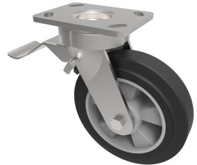
Fabricated swivel castor with a top plate fixing fitted with a black 65 shore A elastic rubber on aluminium centred wheel with ball bearings and a total lock brake. Wheel diameter 100mm, tread width 50mm, overall height 150mm, top plate 150mm x 110mm, hole centres 105mm x 80 or 121mm x 59mm. Load capacity 250kg. REACH compliant also PAH-Free rubber to confirm to EU-directive 2005/69/EC
