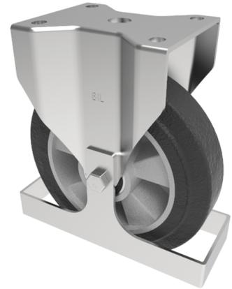
Pressed steel fixed castor with a top plate fixing fitted with a black high elastic natural 65 shore A rubber tyre on an aluminium centred wheel with ball bearings and footguard. Wheel diameter 200mm, tread width 50mm, overall height 238mm, top plate 135mm x 110mm, hole centres 105mm x 80/75mm. Load capacity 500kg. REACH compliant also PAH-Free rubber to confirm to EU-directive 2005/69/EC
