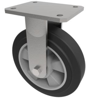
Fabricated white zinc ROHS plated fixed castor with a top plate fixing fitted with a black high elastic natural 65 shore A rubber tyred aluminium centred wheel with a ball bearings. Wheel diameter 200mm, tread width 50mm, overall height 240mm, top plate 138mm x 110mm, hole centres 105mm x 80/75mm. Load capacity 500kg. REACH compliant also PAH-Free rubber to confirm to EU-directive 2005/69/EC \*\* FOR INTERNAL TOWING USE ONLY \*\*
