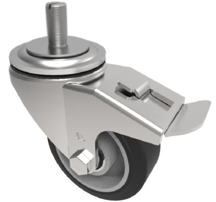
Pressed steel swivel castor with a 12mm bolt hole fitted with a black high elastic natural 65 shore A rubber tyred aluminium centred wheel with ball bearings and total lock brake and fitted with a 16mm x 30mm threaded stem Wheel diameter 100mm, tread width 40mm, overall height 128mm. Load capacity 200kg REACH compliant also PAH-Free rubber to confirm to EU-directive 2005/69/EC
