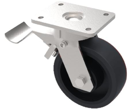
Fabricated swivel castor with a top plate fixing fitted with a black elastic rubber wheel on a cast iron centre with ball bearings and a total lock brake. Wheel diameter 250mm, tread width 75mm, overall height 314mm, top plate 175mm x 140mm, hole centres 140mm x 105mm. Load capacity 750kg.
