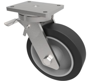
Fabricated swivel castor with a flat plate fixing fitted with a black elastic rubber tyred cast iron centred wheel with ball bearing and total lock brake. Wheel diameter 250mm, tread width 50mm, overall height 314mm, plate size 175mm x 140mm, hole centres 140mm x 105mm. Load capacity 550kg at 4kph \*\* FOR INTERNAL AND EXTERNAL TOWING USE\*\*
