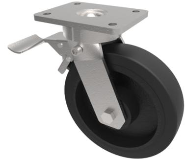
Fabricated swivel castor with a top plate fixing fitted with a black elastic rubber wheel on a cast iron centre with ball bearings and total lock brake. Wheel diameter 200mm, tread width 50mm, overall height 245mm, top plate 138mm x 110mm, hole centres 105mm x 80/75mm. Load capacity 450kg. NB the BIL catalogue is incorrect overall height is 245mm.
