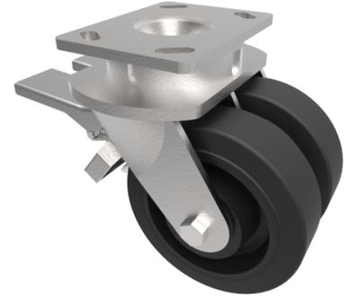
Twin wheeled fabricated swivel castor with a top plate fixing fitted with 2 x elastic rubber tyred cast iron wheels with ball bearings and a double wheel brake. Wheel diameter 150mm, tread width 50mm, overall height 200mm, top plate 150mm x 110mm, hole centers 105mm x 80mm or 121mm x 59mm. Load capacity 700kg.
