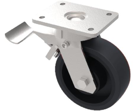
Fabricated swivel castors with a top plate fixing fitted with a black elastic rubber tyred cast iron centred wheel with ball bearings and total lock brake. Wheel diameter 150mm, tread width 50mm, overall height 212mm, top plate 175mm x 140mm, hole centres 140mm x 105mm. Load capacity 400kg at 4kph and 140kg at 20kph. \*\* FOR INTERNAL AND EXTERNAL TOWING USE\*\*
