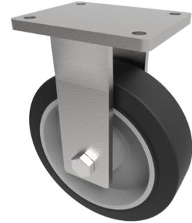
Fabricated fixed castor with a flat plate fixing fitted with a black elastic rubber tyred cast iron centred wheel with ball bearing. Wheel diameter 250mm, tread width 75mm, overall height 314mm, plate size 175mm x 140mm, hole centres 140mm x 105mm. Load capacity 800kg at 4kph and 280kg at 20kph. \*\*
