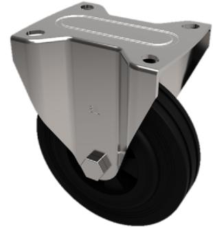
Grade 304 Stainless steel fixed castor with a top plate fixing fitted with a black phenolic wheel with plain bore. Wheel diameter 100mm, tread width 38mm, overall height 133mm, top plate 100mm x 85mm, hole centres 80mm x 60mm or 75mm x 45mm. Load capacity 220kg at a maximum temperature of 120c
