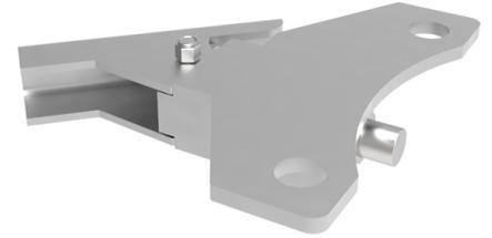
Directional lock for the BZQ series NEW ROCKER STYLE BIL recommend that the lock and the castor are attached to the equipment but before you tighten the nuts totally engage the lock and hammer the lock forward so it totally engages and then tighten the nuts.
