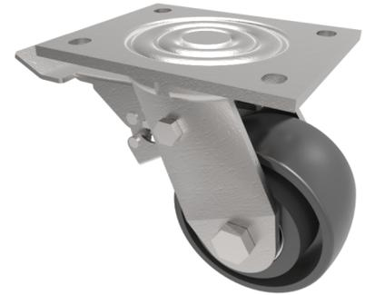
Fabricated swivel castor with a top plate fixing fitted with a black cast iron wheel with a plain bearing with total lock brake. Wheel diameter 100mm, tread width 50mm, overall height 143mm, top plate 135mm x 110mm, hole centres 105mm x 80mm. Load capacity 400kg.
