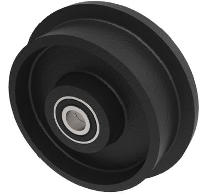
Flanged cast iron wheel with with high temp ball bearings to 270c. Wheel diameter 125mm, outer flange 145mm, tread width 38mm, bore size 20mm, hub length 50mm. tread ascent 3 degrees relative to the wheel axle with a Load capacity 900kg.
