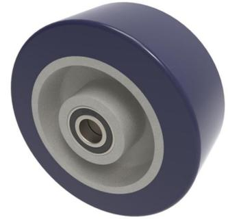
300mm diameter Blue 75 Shore A polyurethane tyre on cast iron centred wheel with ball bearings. Tread width 80mm, bore 25mm, hub 83mm. Load capacity 1,800kg at 4kph and 720kg at 10kph. Also suitable at 630kg at 16kph intermitantly (ask for advise if towing outdoors on tarmac)
