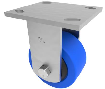
Fabricated fixed castor with a flat plate fixing fitted with 65 shore A blue elastic rubber tyre on a black nylon centred wheel with ball bearings. Wheel diameter 125mm, tread width 50mm, overall height 165mm, top plate 115mm x 102mm, hole centres 92mm x 67mm or 76mm x 76mm, load capacity 275kg. REACH compliant also PAH-Free rubber to confirm to EU-directive 2005/69/EC
