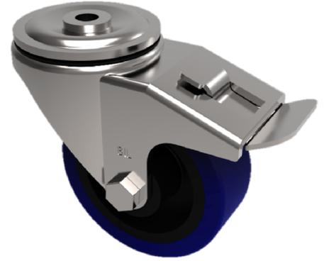
Pressed steel swivel castor with 12mm bolt hole fitted with a 65 shore A blue elastic rubber tyred wheel with a black nylon centre with a plain bore and a total lock brake. Wheel diameter 80mm, Tread width 35mm, Overall Height 110mm, Load Capacity 150kg. REACH compliant also PAH-Free rubber to confirm to EU-directive 2005/69/EC
