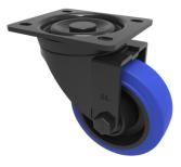
Pressed steel black painted swivel castor fitted with a 65 shore A blue elastic rubber tyre wheel with a black nylon centre with a plain bore. Wheel diameter 80mm, Tread width 35mm, Overall Height 110mm, Top Plate 105mm x 86mm, Hole Centres 80mm x 60mm, Load Capacity 150kg. REACH compliant also PAH-Free rubber to confirm to EU-directive 2005/69/EC
