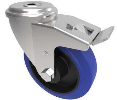
Pressed steel swivel castor with 12mm bolt hole fitted with a 65 Shore A blue elastic rubber tyre on black nylon centre with roller bearings. Wheel diameter 125mm, tread width 36mm, overall height 155mm, Load capacity 250kg. REACH compliant also PAH-Free rubber to confirm to EU-directive 2005/69/EC
