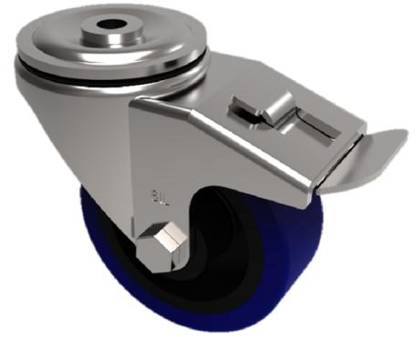
Grade 304 Pressed stainless steel swivel castor with a 12mm bolt hole fixing fitted with a blue 65 shore A elastic rubber tyre on black nylon centred wheel with a roller bearing and swivel wheel brake. Wheel diameter 100mm, tread width 32mm, overall height 128mm. Load capacity 180kg..REACH compliant also PAH-Free rubber to confirm to EU-directive 2005/69/EC
