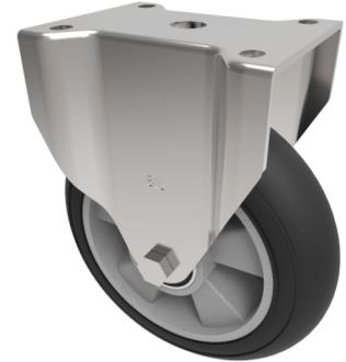
Pressed steel fixed castor with a top plate fixing fitted with a black high elastic natural 55 shore A rubber tyred wheel aluminium centre with ball bearings and total lock brake. Wheel diameter 200mm, tread width 50mm, overall height 238mm, top plate 135mm x 110mm, hole centres 105mm x 80/75mm. Load capacity 380kg at 4kph and 152kph at 10kph. REACH compliant also PAH-Free rubber to confirm to EU-directive 2005/69/EC \*\* FOR INTERNAL TOWING ONLY\*\*
