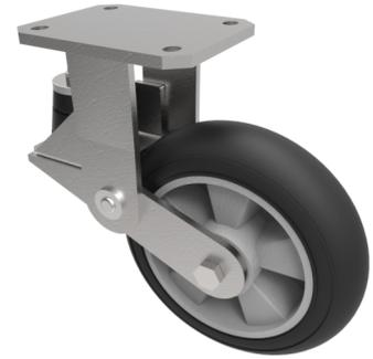
Fabricated fixed castor with top plate fixing fitted with a 200mm x 50mm black ergonomic high elastic natural 55 shore A round profile rubber tyred aluminium centred wheel with ball bearings overall height 237mm/257mm, plate size 138mm x 110mm, hole centres 105mm x 80mm. fitted with a 200kg black rubber spring but load capacity is 200kg at 4kph and 152kg at 10kph. REACH compliant also PAH-Free rubber to confirm to EU-directive 2005/69/EC, also available with flat tread details on request
